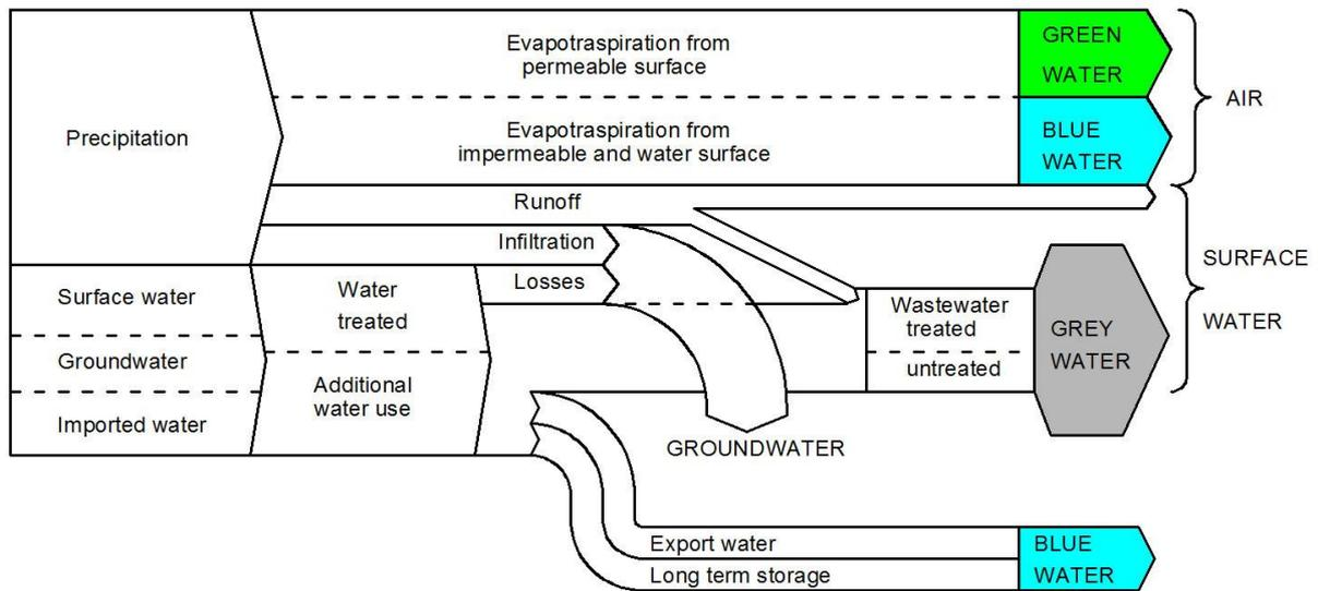
Figure 6: Real water fluxes in the urban area
